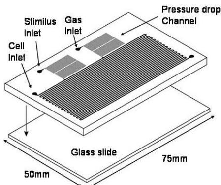
Figure 1. Schematic of the microfluidic system, with inlets for microcarrier introduction, cell stimulus and a gas inlet that can be used to form segmented gas-liquid flow. The main channel is  $300\mu\text{m}$  wide,  $200\mu\text{m}$  deep and approximately  $300\text{cm}$  long.
