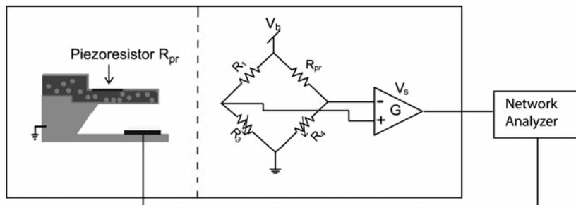
Figure 2: Measurement setup for AC drive of the cantilever and readout from the piezoresistor. The drive signal contains 50VDC and 200mVAC components.
