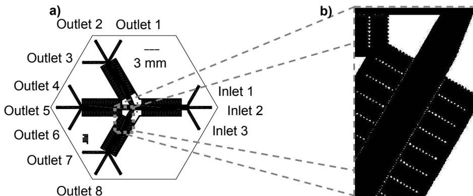
Figure 2: Schematic of multi-stage FF-IEF device.
