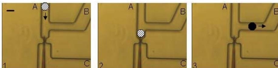
Figure 1: Schematic of microinjection device operation. **Frame 1:** a solution with suspended cells flows into channel A and the suspension fluid is drained thru channel C (the valve in channel C is opened and the valve in channel B is closed). **Frame 2:** a cell reaches the needle, it is pierced and injected. **Frame 3:** The valve in channel C is closed and channel B is opened so that the injected cell is carried away by the fluid.
