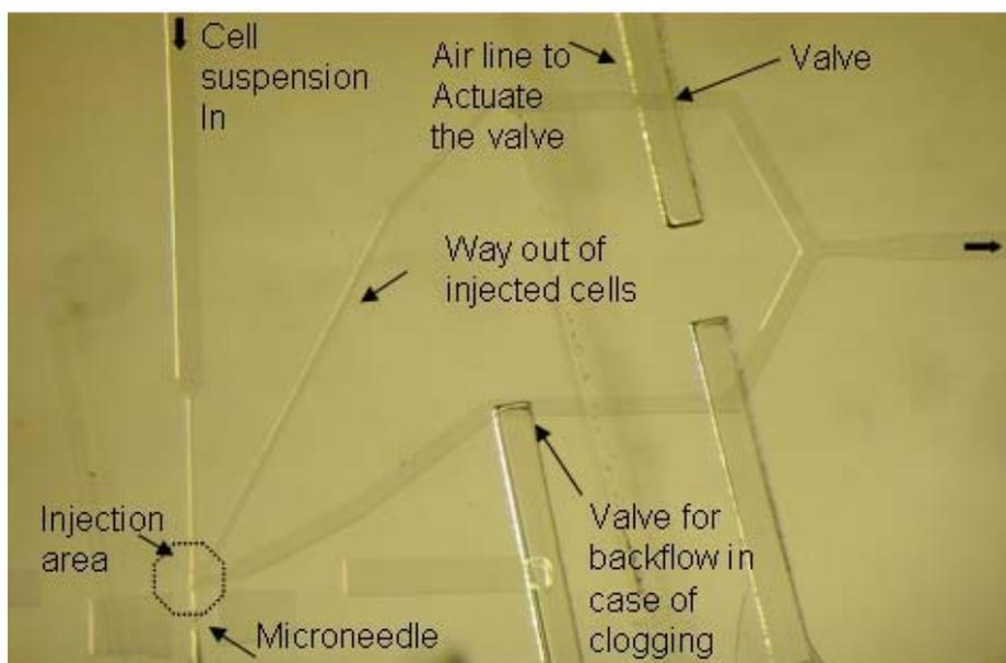
Figure 2: PDMS microfluidic device for single cell microinjection.
