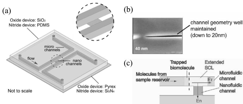
Figure 1. (a) Perspective view of nanofluidic pre-concentrator. Both oxide and nitride devices have 40 nm deep nano channels while 1.5  $\mu\text{m}$  deep  $\mu$ -channel for oxide device, 45  $\mu\text{m}$  for wet-etched device, and 50  $\mu\text{m}$  deep for nitride device. (b) SEM image of the nanochannels. (c) The trapping mechanism.
