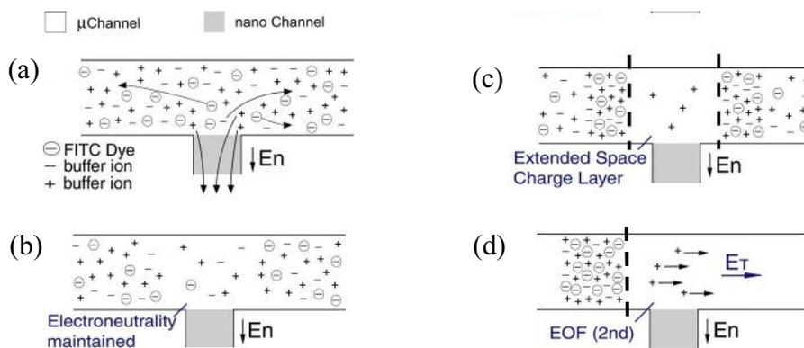
Figure 2. Mechanism of pre-concentration: (a) ion-selective property of the nano channel under small  $E_n$ ; (b) concentration polarization under diffusion-limited condition; (c) at higher field, electroneutrality is no longer maintained, generating an extended space charge layer, (d) With proper  $E_T$  and  $E_n$ , the trapping region and depletion region will be formed as indicated; therefore, samples will be collected in front of the virtual barrier driven by nonlinear electrokinetic flow.
